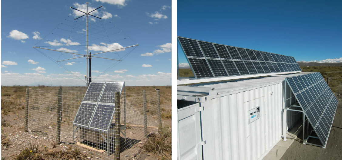
Figure 3.11: ( left ) AERA radio station. ( right ) Central Radio Station: This container hosts the central data acquisition system.
